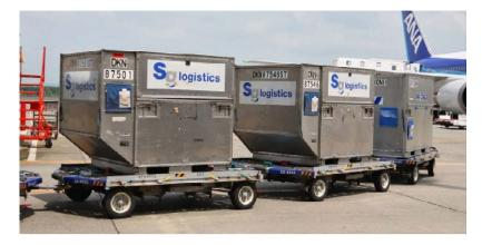
Fig 3.1: Unit Load Devices
